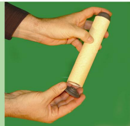
18. Position the top and bottom filter element caps onto the new filter.
