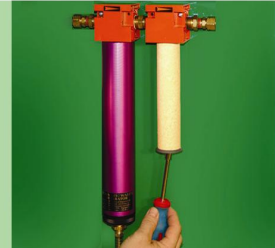
16. Loosen filter element nut using a 5/16" nut driver.
