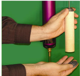
17. Retain the top and bottom filter element caps. Discard old filter.
