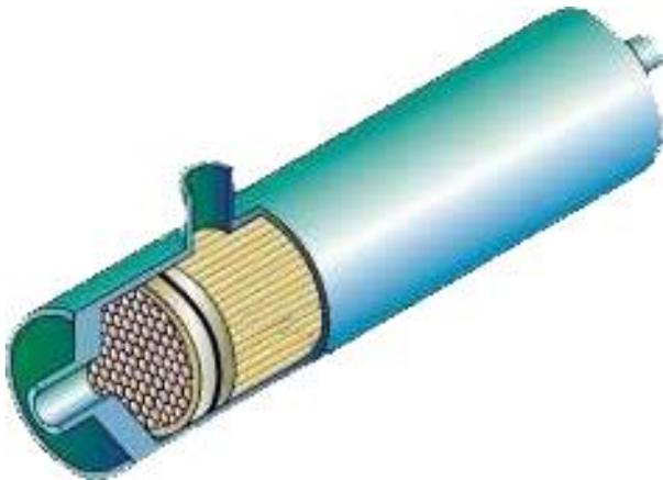
Membrane systems work because nitrogen is a slightly larger molecule than the other components of air. These systems use a semi-permeable membrane that consists of a densely packed bundle of porous tubes. The pores in the tubes are of a size that allows all gases to escape except nitrogen. Compressed air is moved through the membrane and the non-nitrogen gases escape and are vented, producing a constant flow of purified nitrogen.
